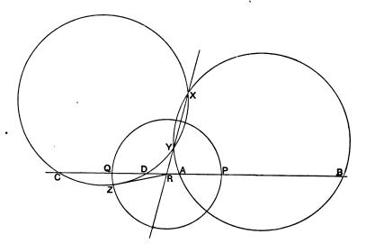
Take any point X not on the straight line, and describe the circles XAB, XCD intersecting again in the point Y.
